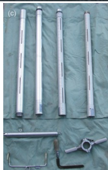
Figure 3. Photograph (a) shows 100- and 33-cm 3 (not used in this study) density cutters; photograph (b) shows 1000- and 250-cm 3 density cutters; and, photograph (c) a Federal snow tube.
