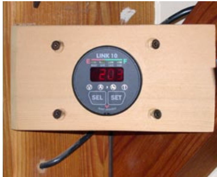
Above: Gauges to measure output from micro hydro generator
