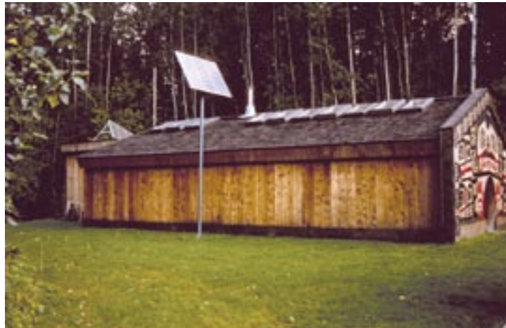
Above: Solar panels and sky lights used to light building
