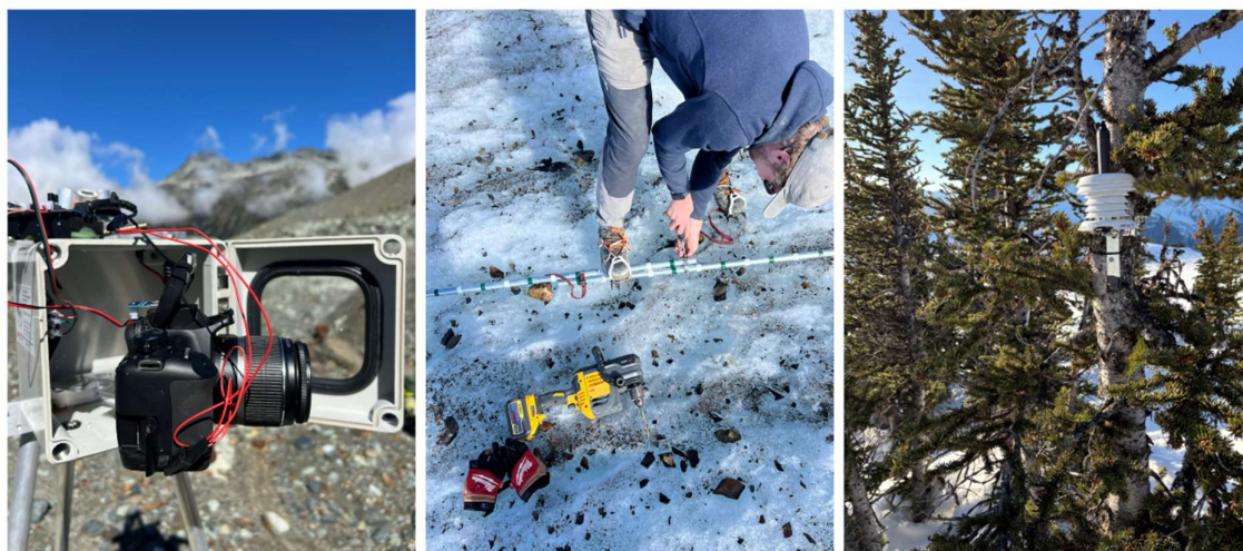
Figure 9. Left: Western timelapse camera setup. Centre: Jeffrey Crompton from the Geological Survey of Canada/Natural Resources Canada securing two sections of an ablation pole together. Right: Barologger installed in January near Overlord Glacier. Image credit: Chloé Monty (left & centre), Iain Sherriff-Scott (right).
