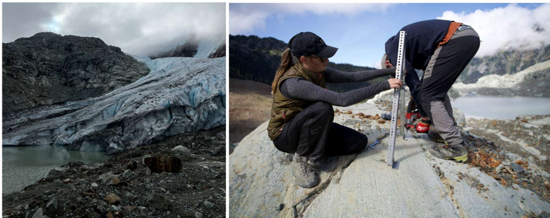
Figure 8. Left: Overlord Glacier terminus in proglacial lake. Right: SFU graduate student Chloé Monty and Jeffrey Crompton from the Geological Survey of Canada/Natural Resources Canada installing a tripod for one of the new time-lapse cameras overlooking the glacier terminus. Image credit: Chloé Monty (left) and Corey Green (right).
