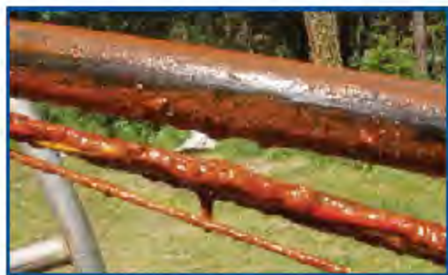
Figure 3. Biofilm on well wiring
