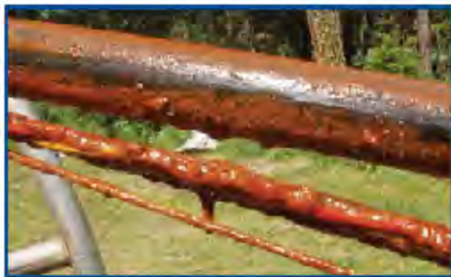
Figure 3. Biofilm on well wiring
