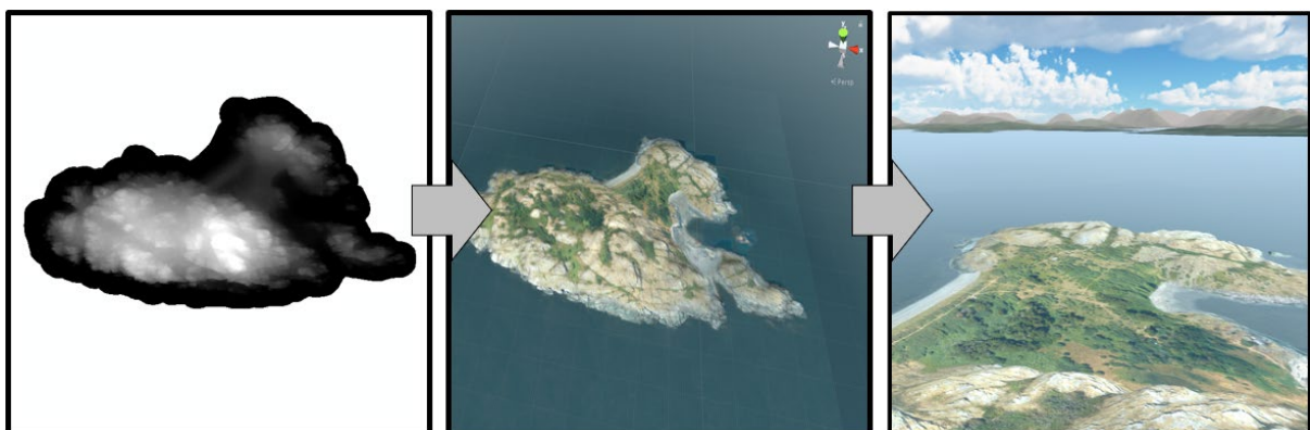
Figure 4. Workflow for developing visualization, from ArcGIS to Unity 3D game engine
