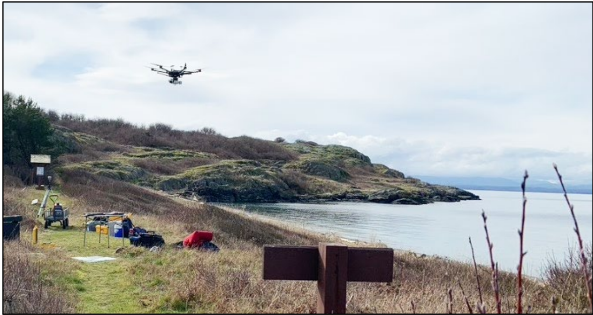
Figure 6. Drone flight conducted on Mitlenatch Island for collecting LiDAR and orthophoto data
