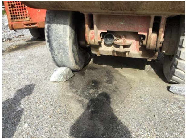
Photo 14: Spill under rock trucks at Tel portal
