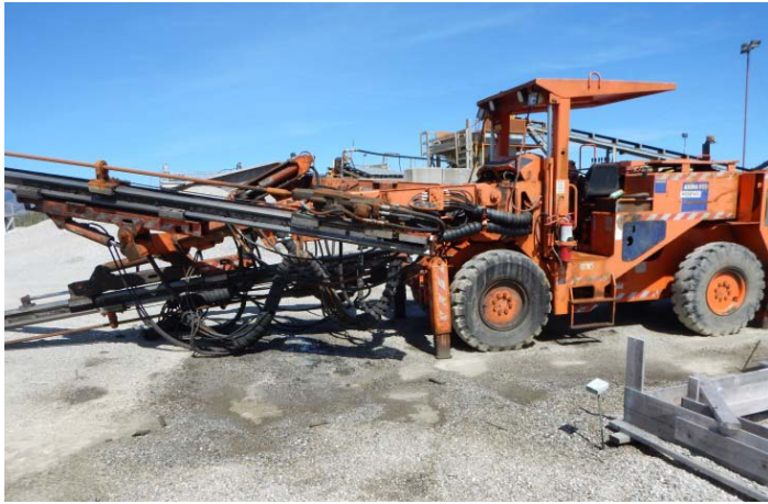
Photo 13: Fluids leaking from drill near truck shop
