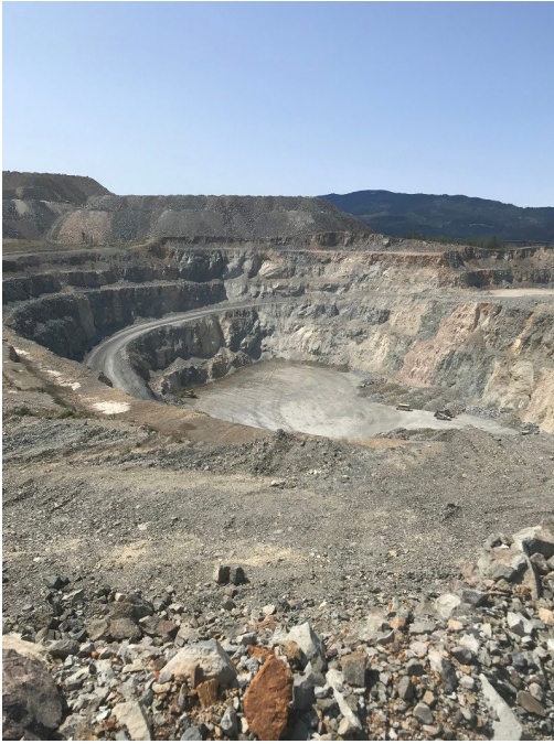
Oriole Pit is currently being backfilled with waste rock
