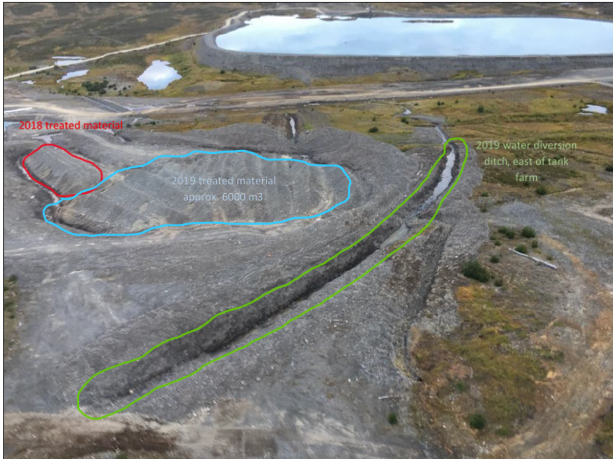
Photo 3.1-2: Aerial View of the In-situ Hydrocarbon Remediation Area - Hydrocarbon Contaminated Soil Treatment.
