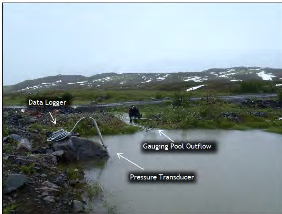
Photo 2.3-1: Hydrometric monitoring station JTS-H1 (tailings storage seepage). August 20, 2019.
