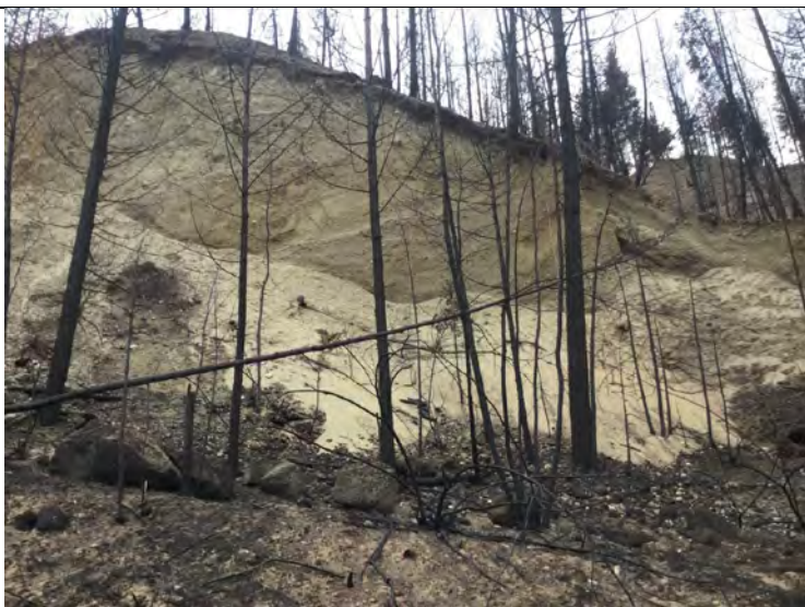
Photo 16: Stratified glaciofluvial and glaciolacustrine sediments exposed along side slopes above water pipeline and Lambly Creek (Bear Ck Rd-2)
