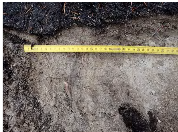
Photo 19. TP20. After >40 seconds, 100% of drops not infiltrating. See 10 cm intervals.
