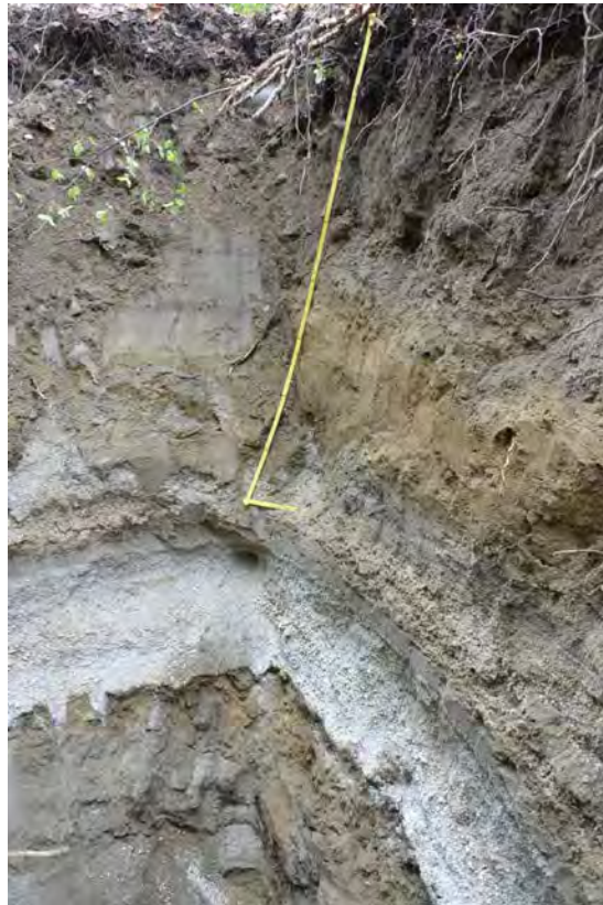
Photo 8. Bridge River tephra, 200-250 cm depth, buried by reworked tephra, and two debris flood units (sand/fine gravel), Walker Creek fan. (Cordilleran 2015).
