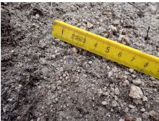
Photo 3. Bridge River tephra grain size, 1-10 mm diameter, sand to granule gravel.
