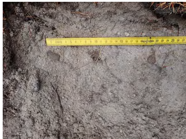
Photo 17. TP19. After >40 seconds, 50% of drops not infiltrating. See 10 cm intervals.
