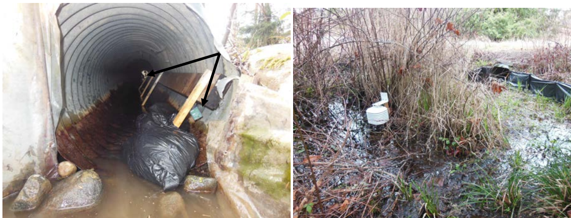
Photo 72. Passive data loggers installed in (one at the mouth and one 15 m inside; black arrows) and outside of culverts to compare internal versus ambient air temperature. Photo credit: Elke Wind.
