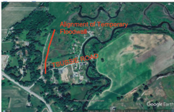
Photo 12: Alignment of Temporary Flood Wall Partially Protecting Tsussie Road
