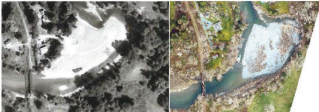
Photo 10: Air photos from 1992 (left) and 2021 (right) showing how channel morphology has changed in the depositional area over time
