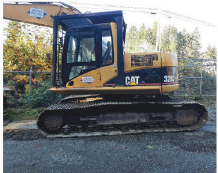
Photo 7: Excavator arriving on site pressure washed clean to avoid introduction of invasive species.
