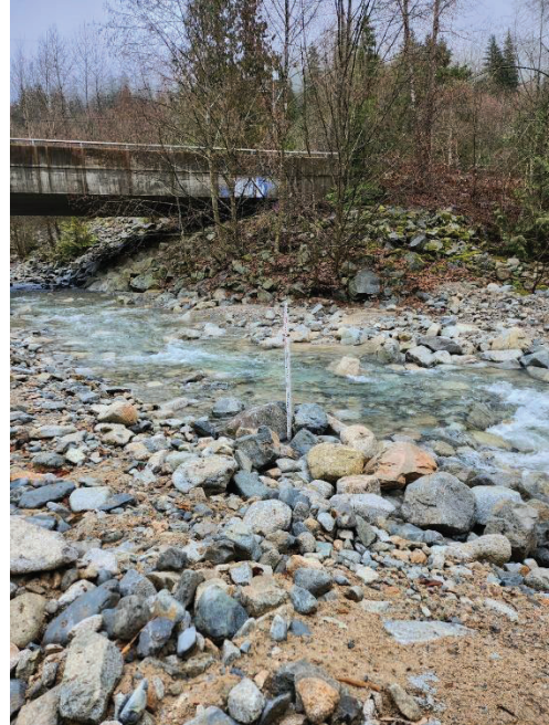
PHOTO #4 – Water meter placed below bridge to observe water level
