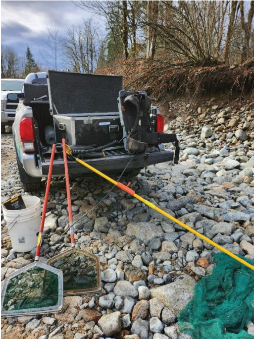
PHOTO #3 – Electro-fisher, seine net/fence and fish salvage equipment
