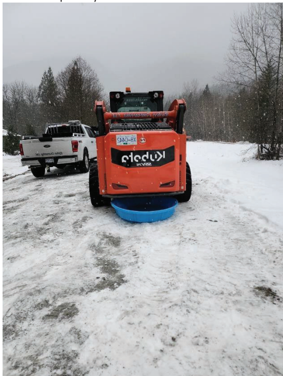
PHOTO #3 – Spill-tray under skid steer
