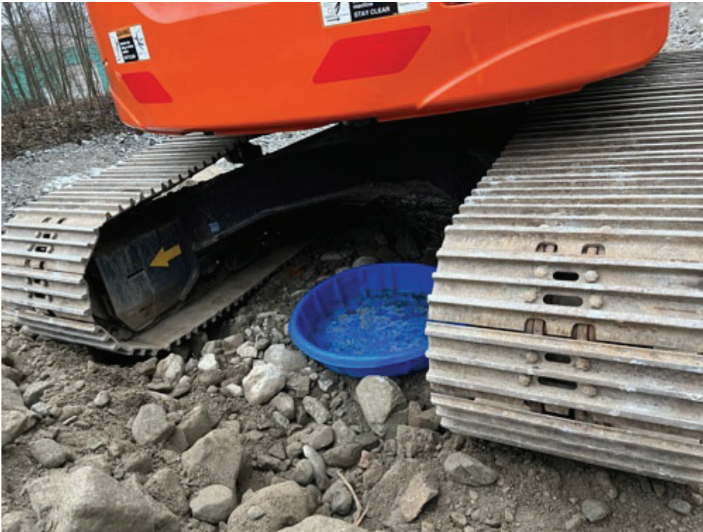
Photo 2. Drip trays underneath machinery.
