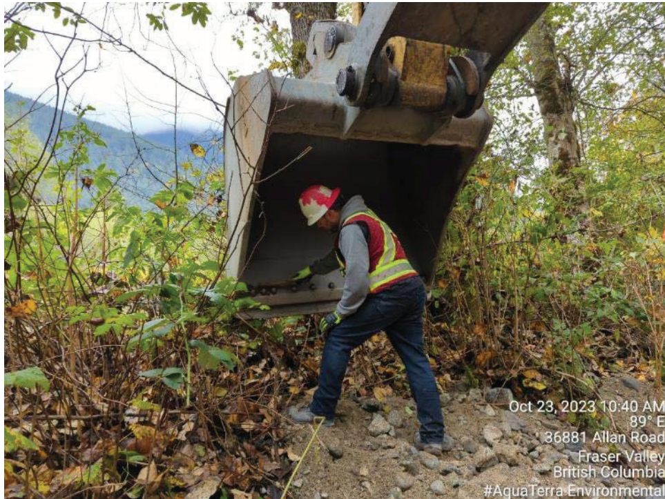
Photo 6: Excavator bucket cleaned with stiff metal brush.
