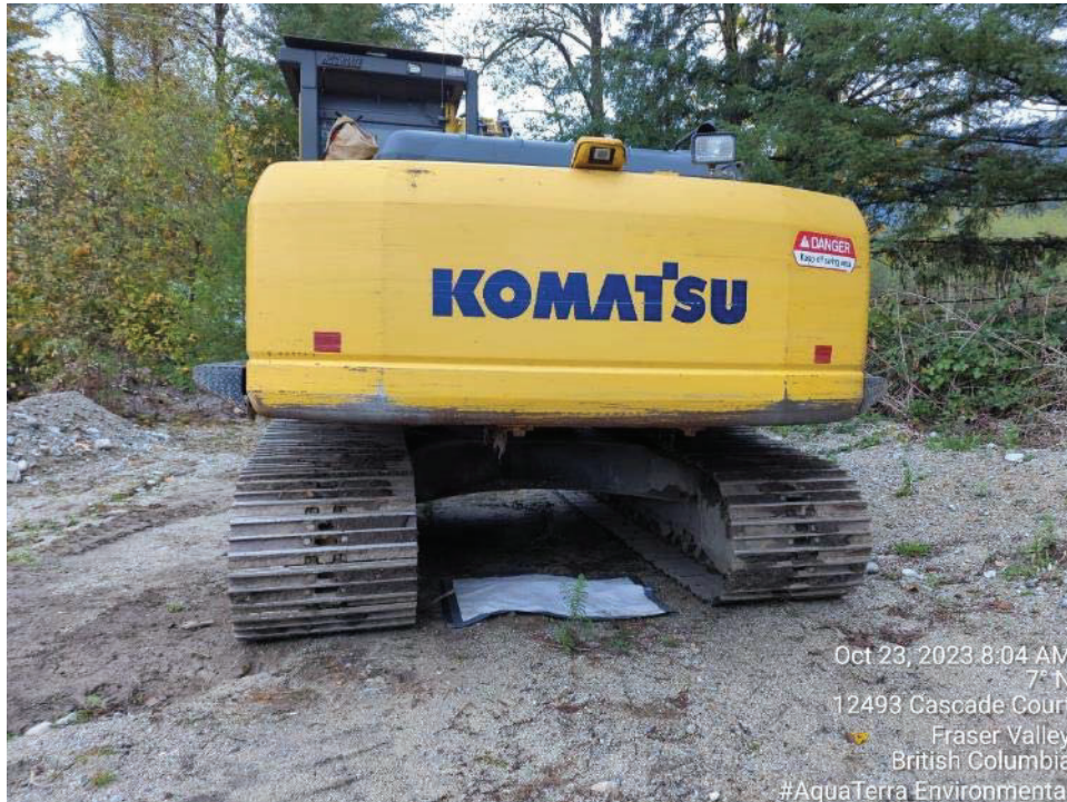
Photo 2: Drip pad observed under inactive excavator.
