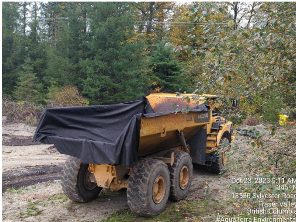
Photo 3: Geotextile fabric lining in the rock truck.
