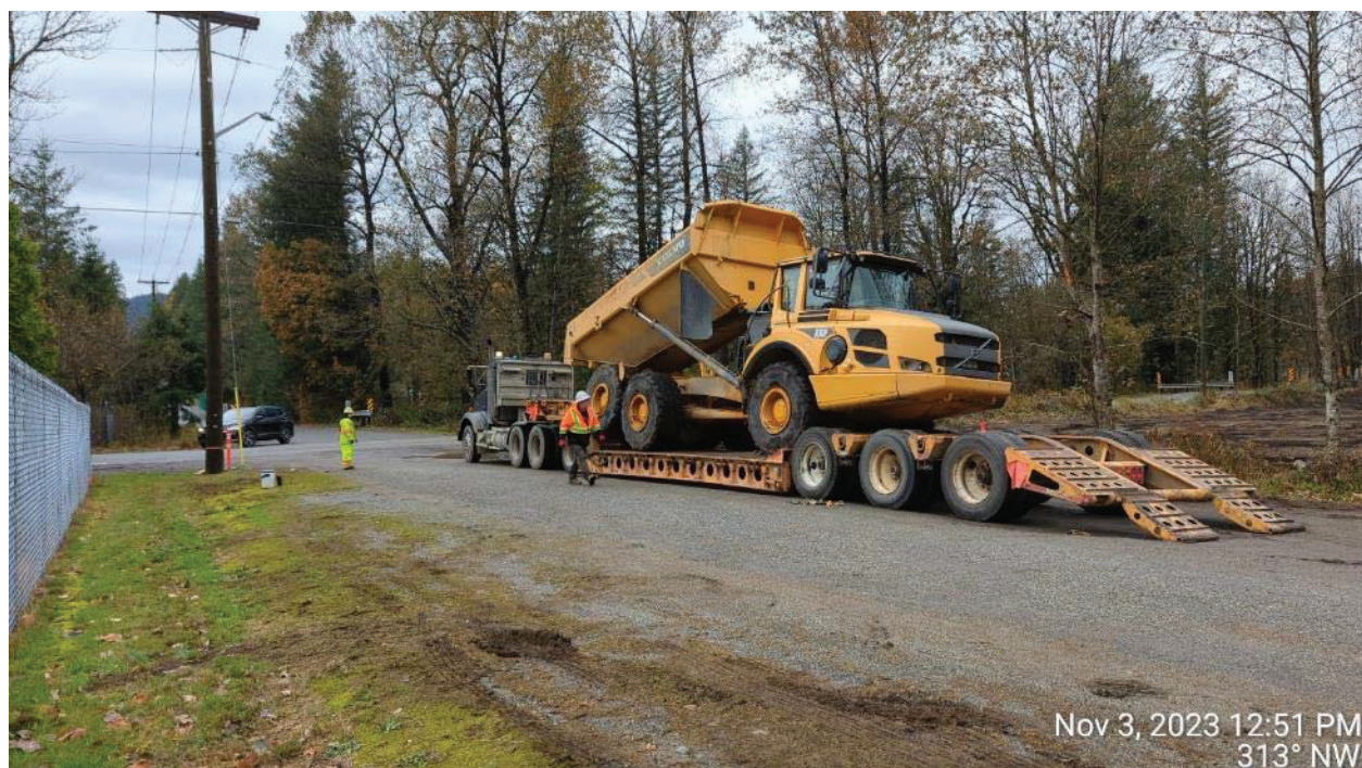
Photo 25: One (1) rock truck loaded onto the flatbed for removal.
