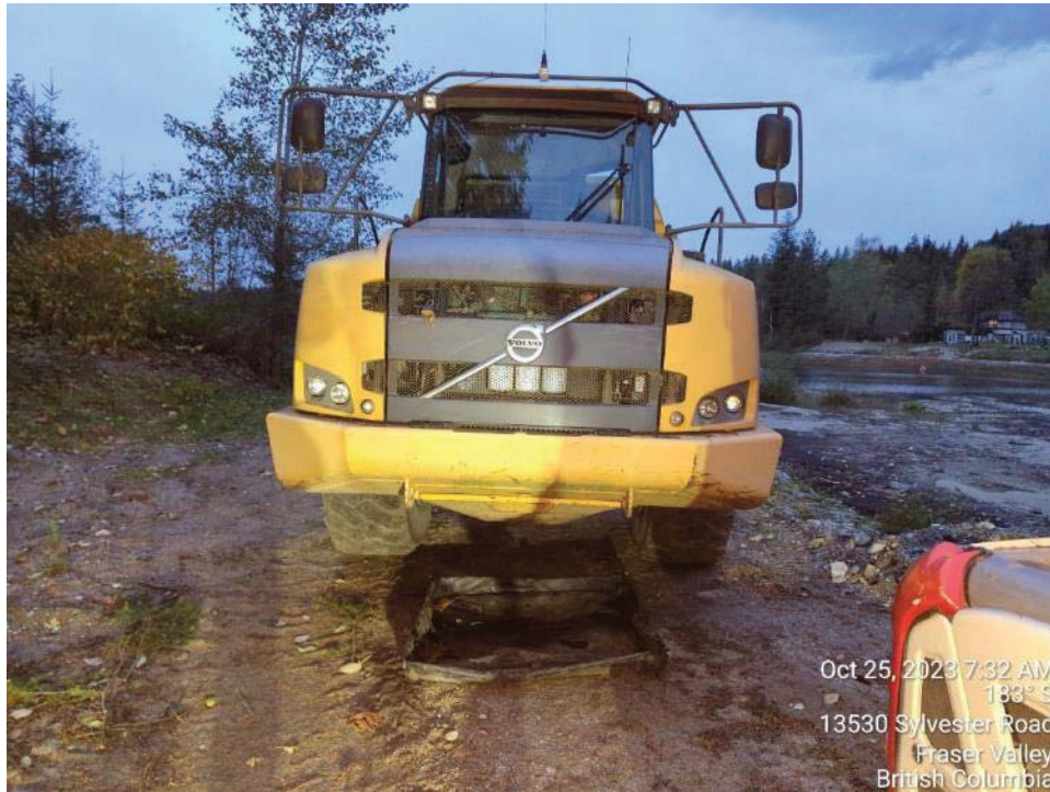
Photo 8: The rock truck adequately protected with a drip tray at the time of inspection.
