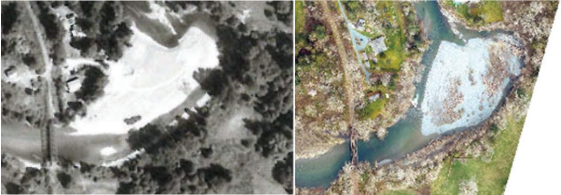
Photo 14– Air photos from 1992 (left) and 2021 (right) showing how channel morphology has changed in the depositional area over time (Source: NHC 2022)
