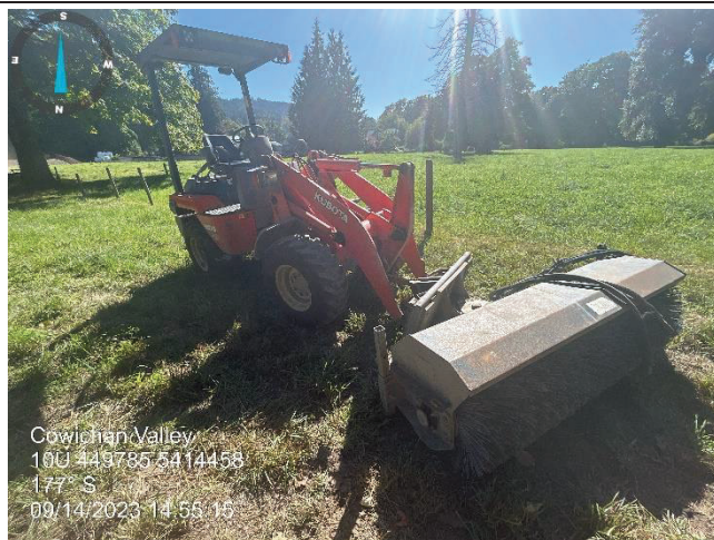
Photo 6: Machine used to clean road at end of shift
