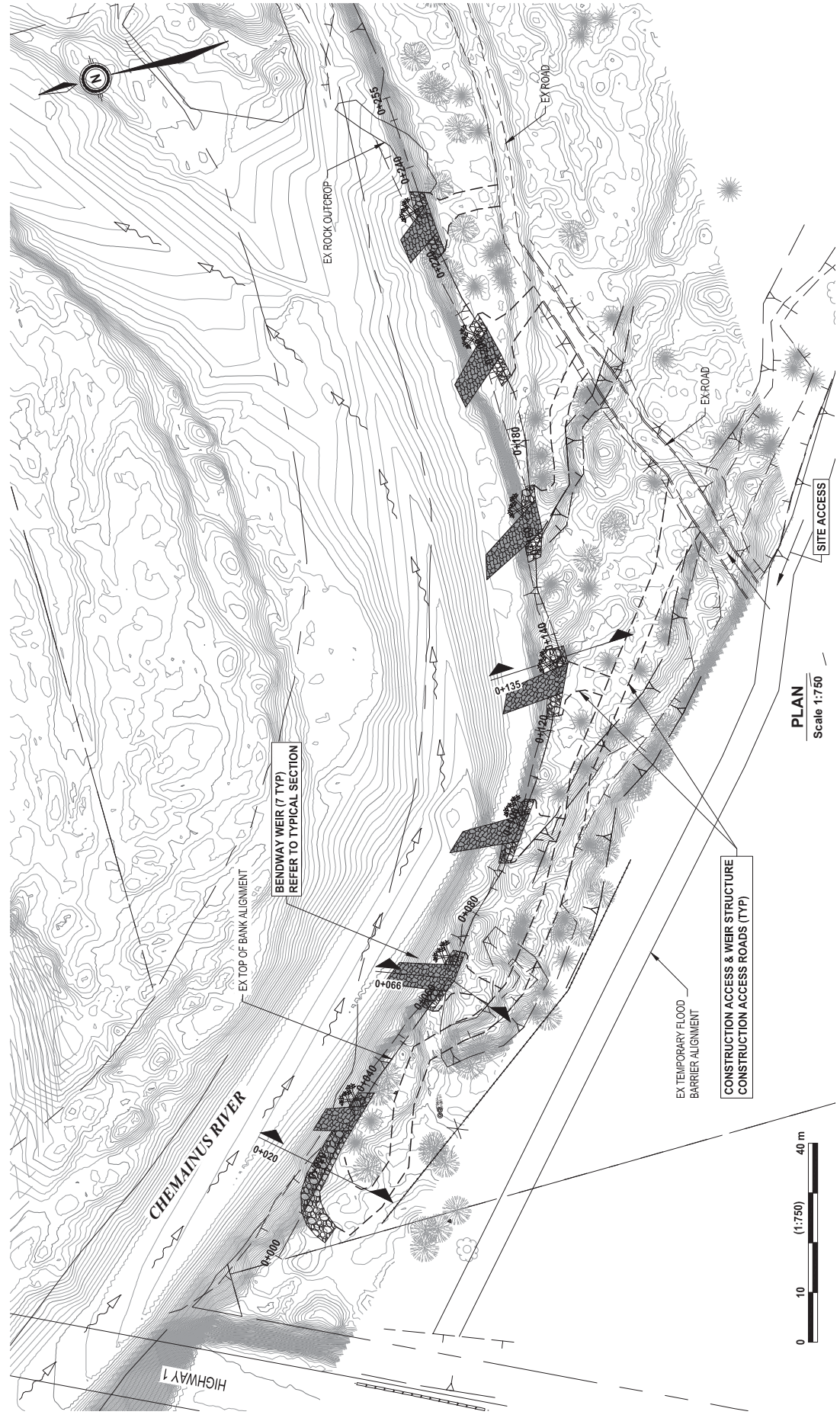
FIGURE A-2 BENDWAY WEIR STRUCTURES CONSTRUCTION PLAN
