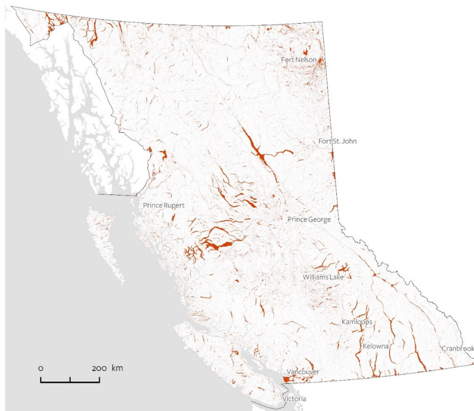
Figure 3-1 Riverine flood hazard where floodplains are based on modelled 1:200-year flood extents for a minimum catchment area of 10 km 2 (example map of hazard extent).
